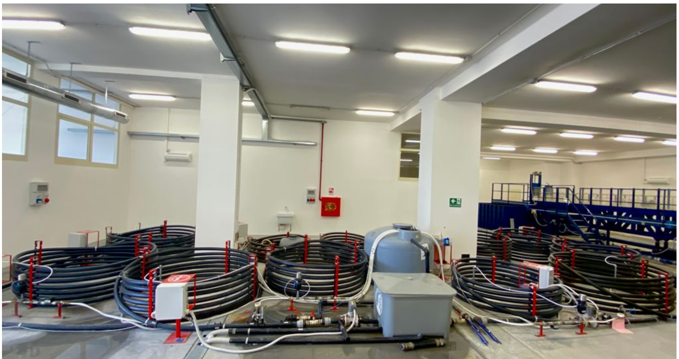
Figure 1. Layout of the water distribution network located in the LIA Laboratory. (a): Schematic representation of the WDN; (b): representation of the real laboratory network.
